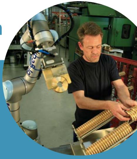
→ If possible, avoid the need for vision systems or sensors to identify and pick up parts. Handling parts with divergent properties (size and shape) or unstructured presentation (jumbled in a bin) can definitely be done, but is more complex.
